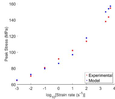
Figure 3: Comparisons of peak stresses for the model predictions and experiments.
